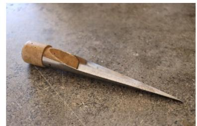
Figure 90 Poinçon creux
