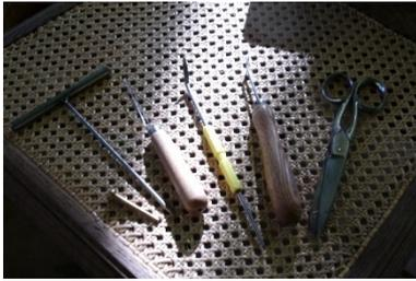
Figure 94 Cheville, pointes à tracer, tire cane, ciseaux
