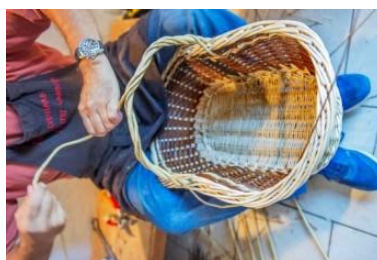
Figure 131 - Cordelage des brins
